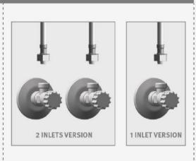
MAKE SURE THAT THE FILTER(S) IS/ARE INSTALLED BETWEEN THE FLEXIBLE PIPE AND THE SHUT OFF VALVE (ANGLE VALVE) (NOT SUPPLIED).
